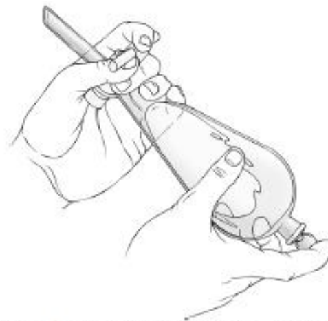
Figure 12.6 The correct way of shaking and venting a separatory funnel.
