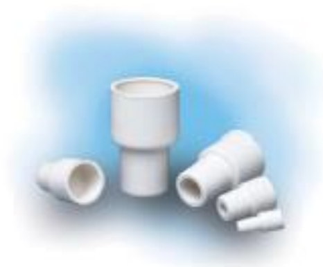
Figure 4.13 Rubber septa for some of the most common sizes of ground-glass joints. © Sigma-Aldrich Co. The narrow, hard end is inserted into the joint and the wide, more flexible end is folded down over the outside of the joint.
