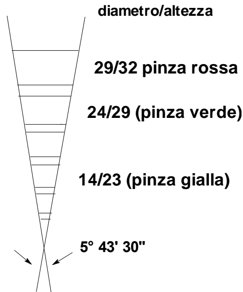
Fig. 17 Standard taper joints (ISO 19/22).
