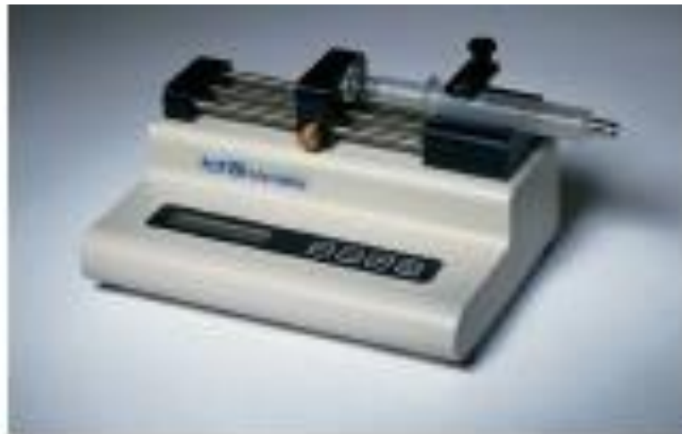
Figure 4.15 A syringe pump accepts a variety of sizes of syringes and drives a ram against the plunger at a constant rate. The rate of liquid delivery is variable based on the size of the syringe and the setting of the syringe pump.
