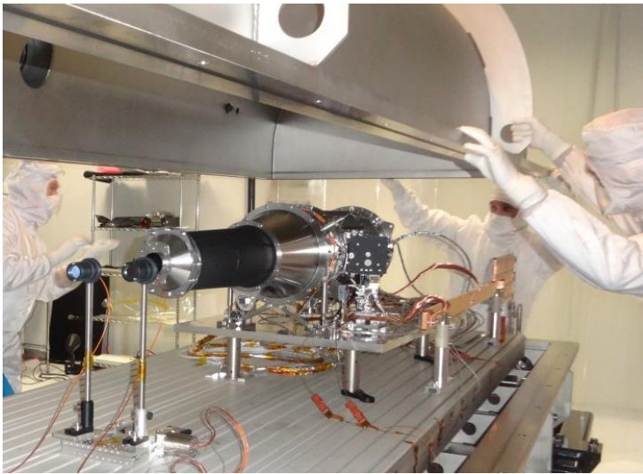
Metis just before initiation of pumping for calibration with the UV source (ALENIA Turin, March 25, 2017)
