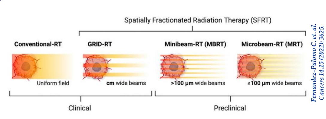
**MINIBEAM EFFECT:** Reduction of damages to normal tissues due to the spatial fractionation of the dose while maintaining a homogeneous coverage of the tumour volume.
